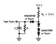
C = 30 pF for BA, BS 130 pF for D0-D7, E, Q 90 pF for A0-A15, R/W
