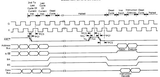
NOTE: Waveform measurements for all inputs and outputs are specified at logic high 2.0 V and logic low 0.8 V unless otherwise specified
