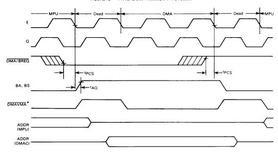
FIGURE 14 — AUTO-REFRESH DMA TIMING (>14 CYCLES) (REVERSE CYCLE STEALING)
